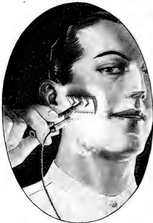
A miniature electric lamp is attached to the handle of the safety razor and helps to illuminate the gentle art of shaving
